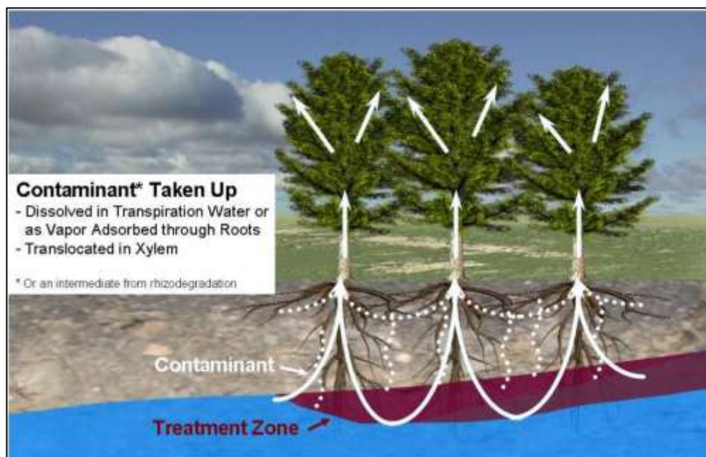
Figure 6. Phytoextraction Mechanisms to Capture Soil and Groundwater Contaminants [8].
